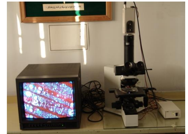
Projection Microscope with Scanning, Saving, and Image Analysis Capabilities
